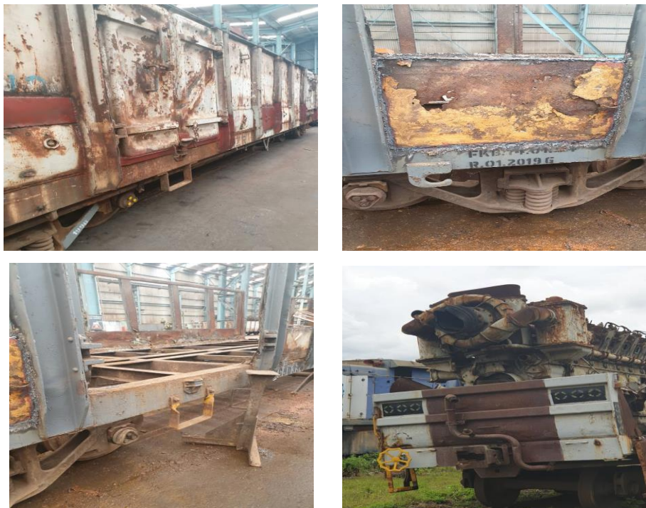
Figure 23.4: Poorly maintained wagons and other rolling stock
