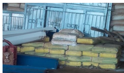
Hardened bags of cement
