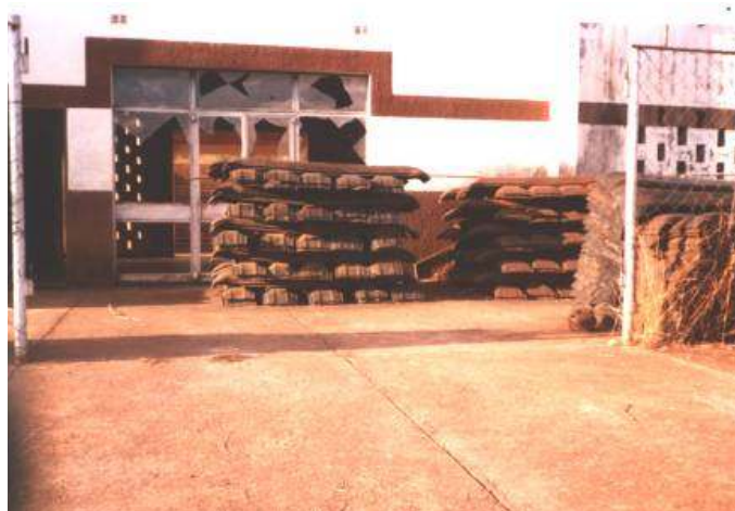
Unused steel sleepers stockpiled at the station.
