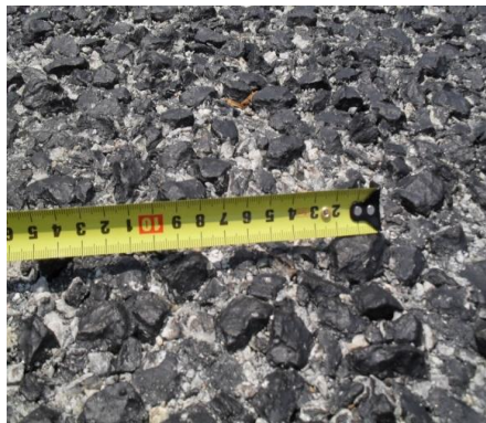
Second layer aggregates sizes
