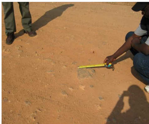
Over sized stones contained in the gravel at KM2.4
