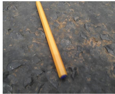
Big aggregate particles used for surface dressing
