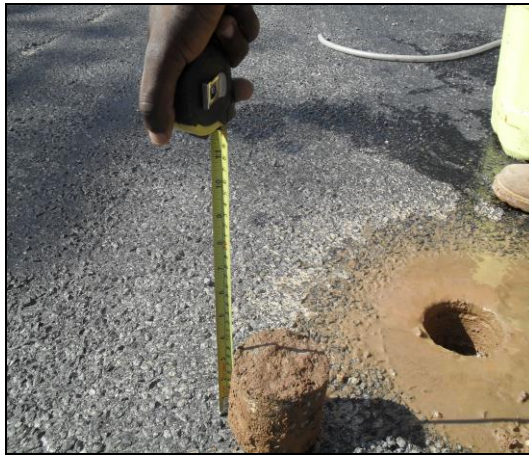
Sample reading 80mm as opposed to 150mm paid by the Government
