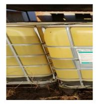
Container at half its contents due to spillage
